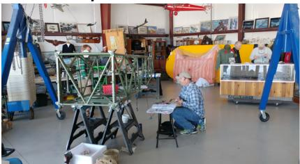
Work on the Stearman continues to be slow but steady. Over the last month, control cables and various other components have been reinstalled in the frame. Almost all components have been cleaned, blasted, and repainted.
